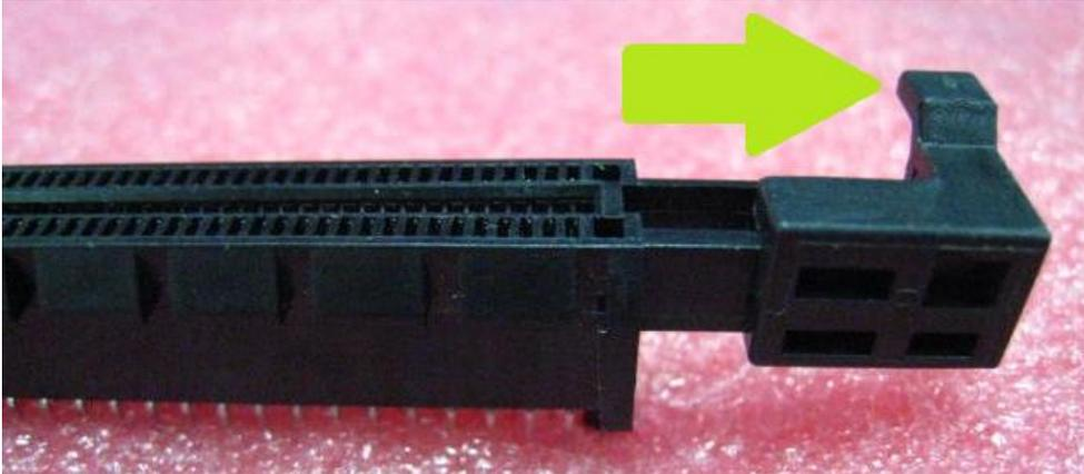
2. After install VGA card, please move the lock back to the Locked position.
